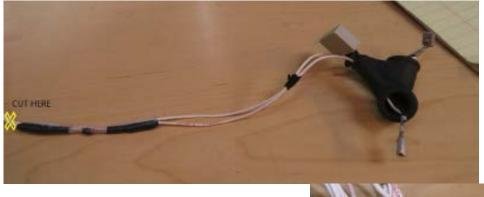
Install female connector (supplied) to X3 harness wire labeled XS34.
