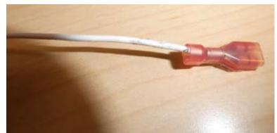
Install male connector (supplied) to X3 harness wire labeled XS35.
